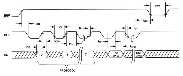
NOTE:  $t_{CL}$ ,  $t_{CH}$ ,  $t_{R}$ , and  $t_{F}$  apply to both read and write data transfer.
