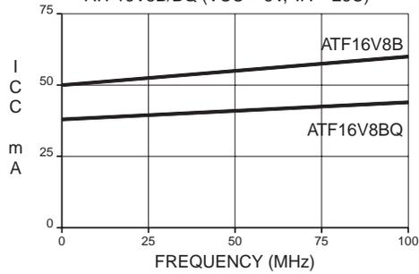
**SUPPLY CURRENT vs. INPUT FREQUENCY**
