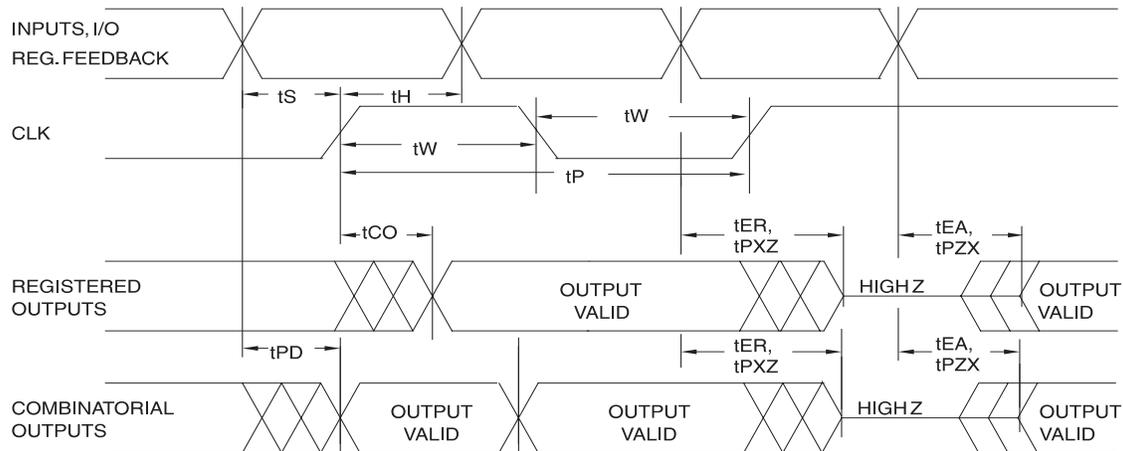
Note: 1. Timing measurement reference is 1.5V. Input AC driving levels are 0.0V 3.0V, unless otherwise specified.
